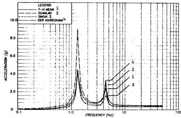
FIG. 9 - BUILDING MODEL : SINGH, DER KIUREGHIAN, & SCANLAN SPECTRA
