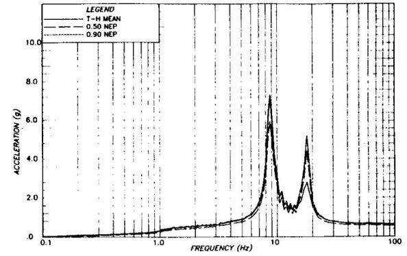
FIG. 8 - CONTROL PANEL MODEL : T-H MEAN AND VARIOUS NEP LEVELS
