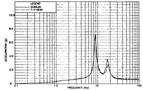
FIG. 10 - CONTROL PANEL MODEL : SCANLAN SPECTRUM AND T-H MEAN
